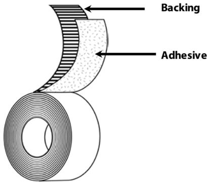
**Backing:** Fiberglass-Reinforced Polypropylene Film
