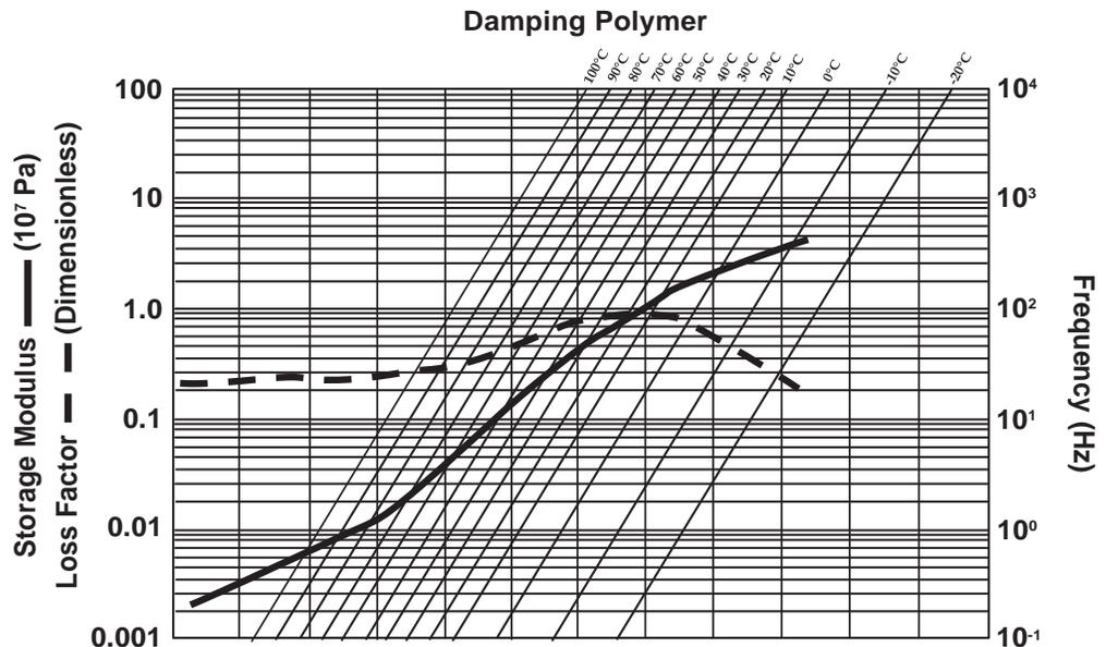
**Test Method:** These properties were determined isothermally at each temperature on a Polymer Laboratories Dynamic Mechanical Thermal Analyzer (DMTA). The strain amplitude used 8.47% peak to peak. Measurements were done at frequencies of 0.3, 1.0, 3.0, 10, and 30 Hz. Data at non-test frequencies and temperatures were determined from time-temperature superposition principles.
